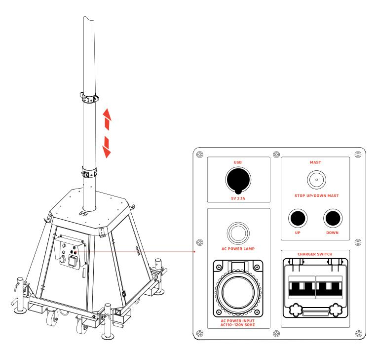
Press the UP and DOWN buttons on the control board to adjust the pole height.
