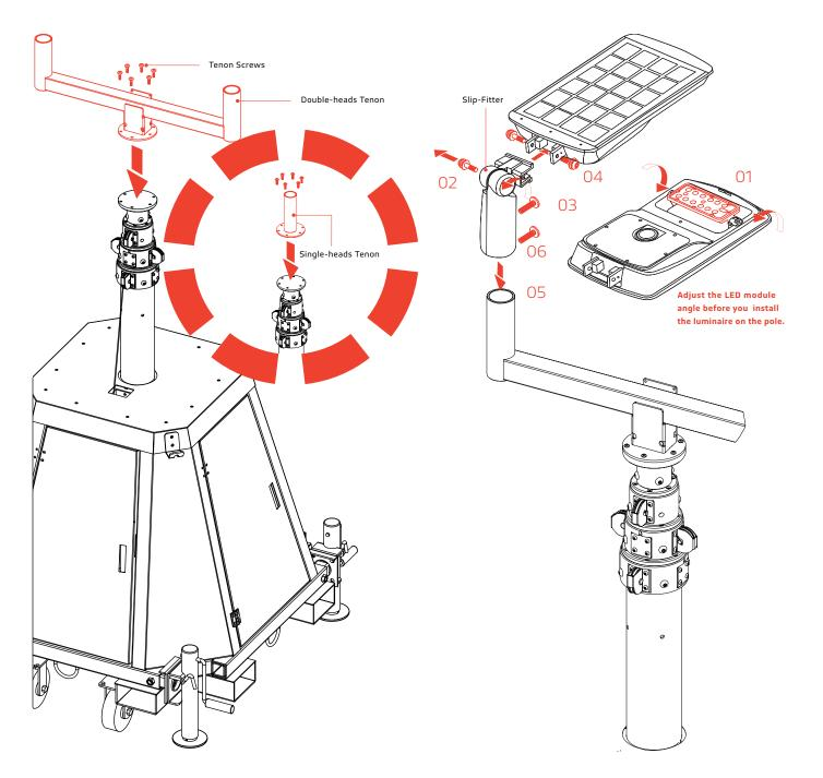
Install Tenon on the top of the pole.
