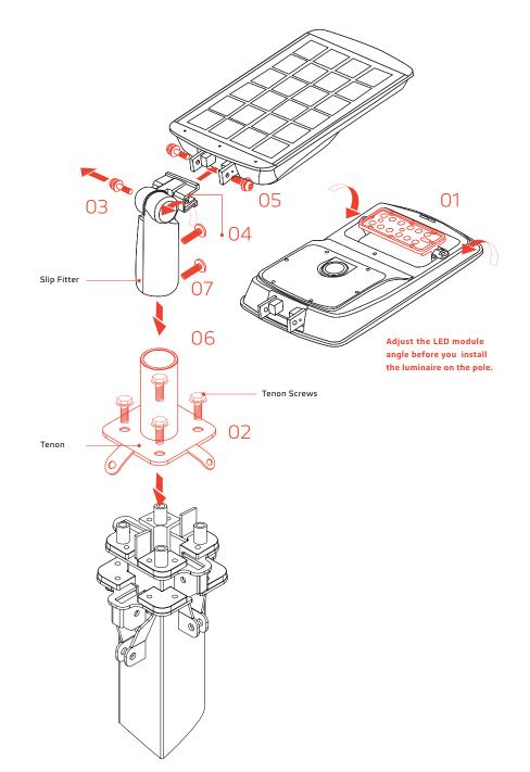
Install Tenon and Luminaire on the top of the pole.
