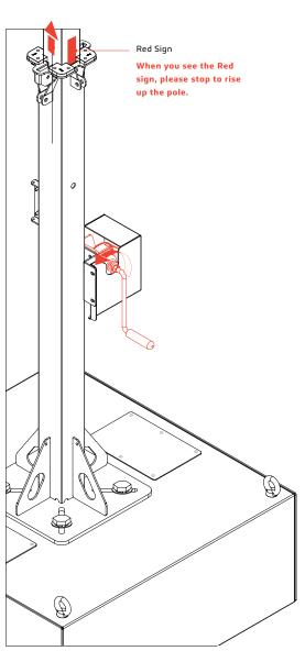
Rotate the handle to adjust the height of the pole.
