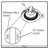
4.) Carefully tuck all wires into junction box and replace the junction box cover panel. Fold up both spring arms and insert the entire fixture up through the ceiling while letting the tension on the spring arm close onto the upper surface of the ceiling panel. Ensure that the fixture is secured to the ceiling before releasing support of the fixture and completing the installation.
