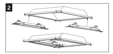
3. Insert the two side bars into the clearance between the brackets and the T-grid.
