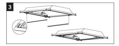
4. Using the included self-tapping screws, use electronic screwdriver to secure brackets into place through bracket mounting holes from inside of the fixture. Caution: Luminaire wiring and electrical parts may be damaged when drilling for installation of LED retrofit kit. Ensure that enclosed wiring and components have not been damaged.
