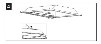
5. Embed the rotary screws on the edge of the panel into the bracket chutes. Push to the end in the direction of chutes to secure panel.
