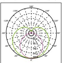
$\begin{array}{l} \text{Maximum Candela} = 1248.55 \\ \text{Located at Horizontal Angle} = 0, \\ \text{Vertical Angle 0} \end{array}$
