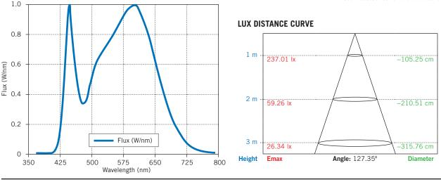
Note: The curves indicate the illuminated area and the average illumination when the luminaire is at a different distance.
