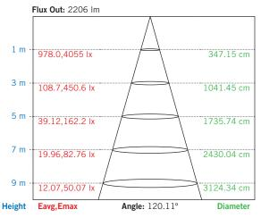
Note: The curves indicate the illuminated area and the average illumination when the luminaire is at a different distance
